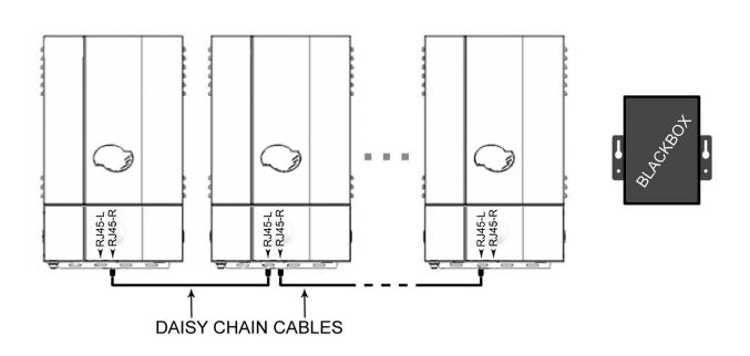
**STEP 4.** Connect the RJ45-L port of each inverter to the RJ45-R port of the next inverter with daisy chain cables as shown.
