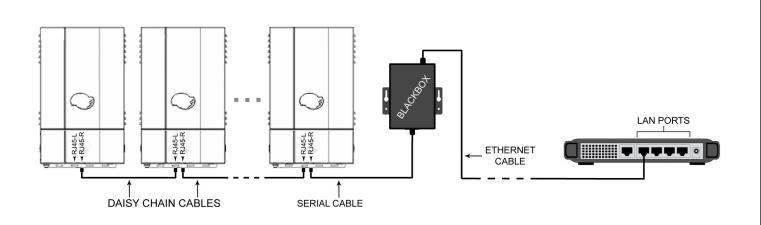
**STEP 6.** Connect ethernet port of Blackbox to any one of the LAN ports (These ports are usually numbered.) on your internet router using a standard CAT 5E ethernet cable. Make sure ethernet cable is not in the way of foot traffic.
