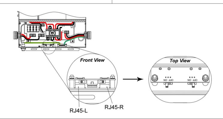
**STEP 3.** Unscrew and remove lower panels of all inverters to reveal switches controlling the comm ports, RJ45-L and RJ45-R, of each inverter.
