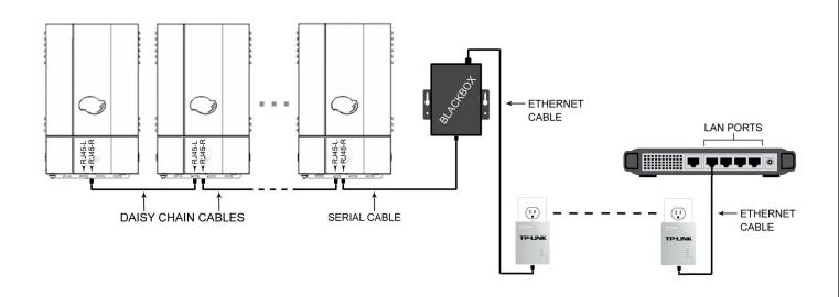
**STEP 6 ALTERNATE.** Connect to ethernet through the TP-LINK powerline adapter, which uses your home's existing wiring. You will still need shorter lengths of CAT 5E ethernet cabling at both ends as shown.
