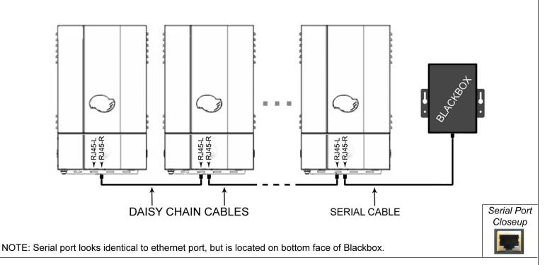
**STEP 5.** Connect RJ45-R comm port of *first* inverter to serial port of Blackbox with serial cable as shown. The end of the serial cable marked "BB" plugs into the Blackbox, while the end of the serial cable marked "INV" plugs into the inverter.
