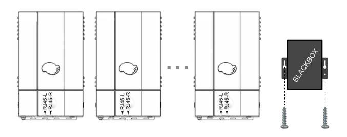
**STEP 2.** Mount Blackbox near the *first* inverter (the same inverter designated as the first inverter in *Part I Step 4* of these instructions) making sure that Blackbox will not be exposed to water or extreme temperatures (below -40C or above 66C).
