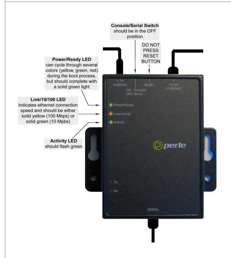
**Step 8.** After power up, allow two minutes for Blackbox to boot. Confirm that LEDs are behaving as described above. If not, check that all connections are made properly. Then unplug and replug Blackbox. After proper LED behavior is confirmed, allow at least 3 hours of sunlight to pass (for data collection) before proceeding to Part III of instructions.
