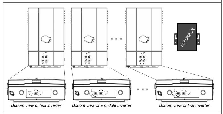
**STEP 3.** On the inverters, unscrew and slide away covers over all comm ports *except* the cover over comm port, RJ45-L of the *last* inverter (the same inverter designated as the last inverter in *Part I Step 4* of these instructions) as shown.
