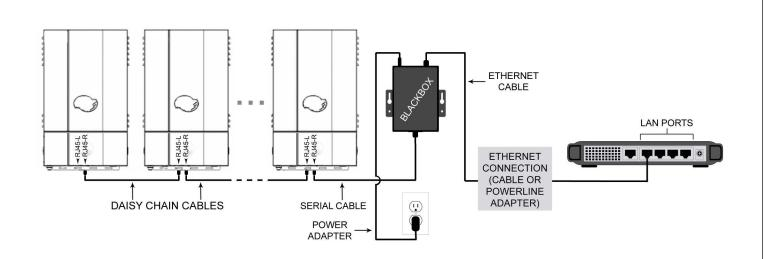
**STEP 7.** Power up Blackbox by plugging it into a standard 110V outlet with the power adapter.
