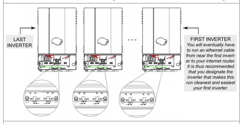
**STEP 4.** On the *last* inverter, set the RJ45-L switch to ON and the RJ45-R switch to OFF as shown. Set all other switches of all other inverters to OFF as shown. Refasten lower panels of all inverters.
